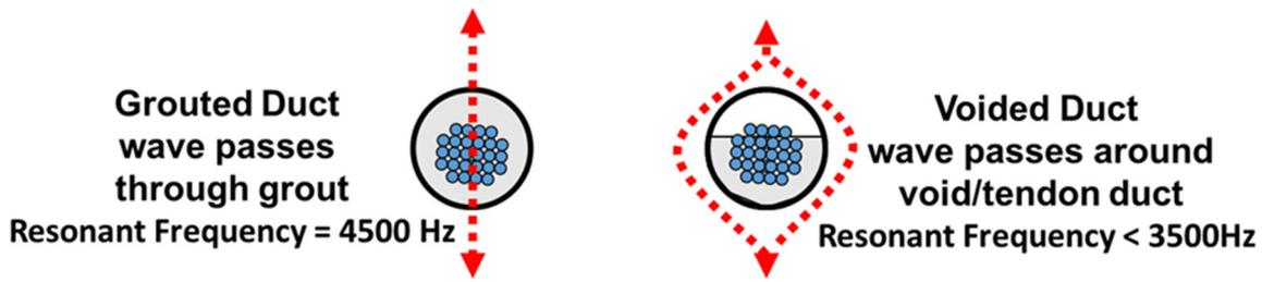
Figure 6: Sonic Wave Paths for fully Grouted and Voided Ducts
